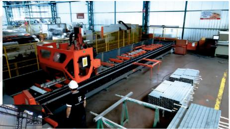
We have a total of 7 CNC machines, Including 3 of 5 axis CNC , 3 of CNC 4 axes , 1 of CNC 3 axes.
